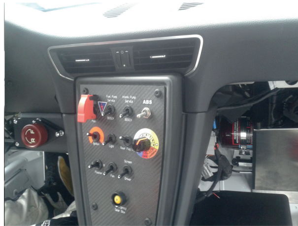
Illustration 22: ABS On/Off and ABS 12-position switch
