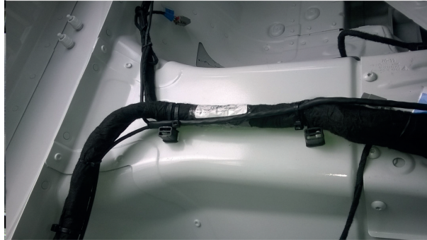
Illustration 25: ABS loom on top of center tunnel
