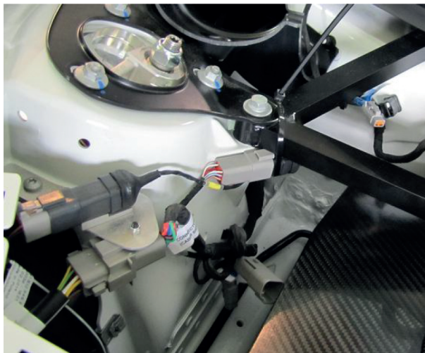
Illustration 15: ABS loom connected
