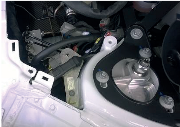
Illustration 13: Wiring loom position at ABS exit
