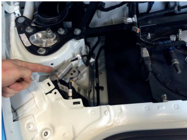
Illustration 14: Wheel speed sensor FR connector w/o ABS
