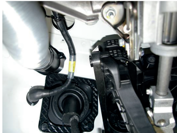
Illustration 23: ABS loom runs from connection point upwards
